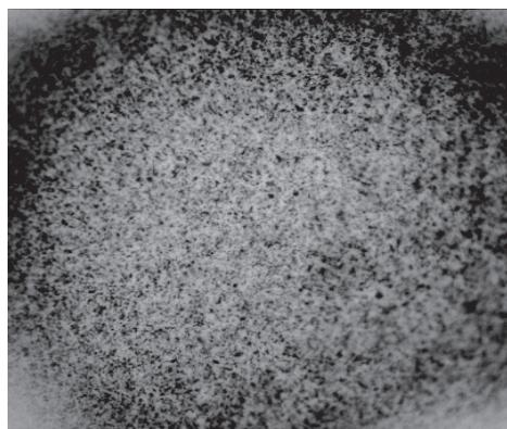
Fig. 2 Typical optical micrograph of speckle pattern on  $\text{Al}_2\text{O}_3$  surface.
